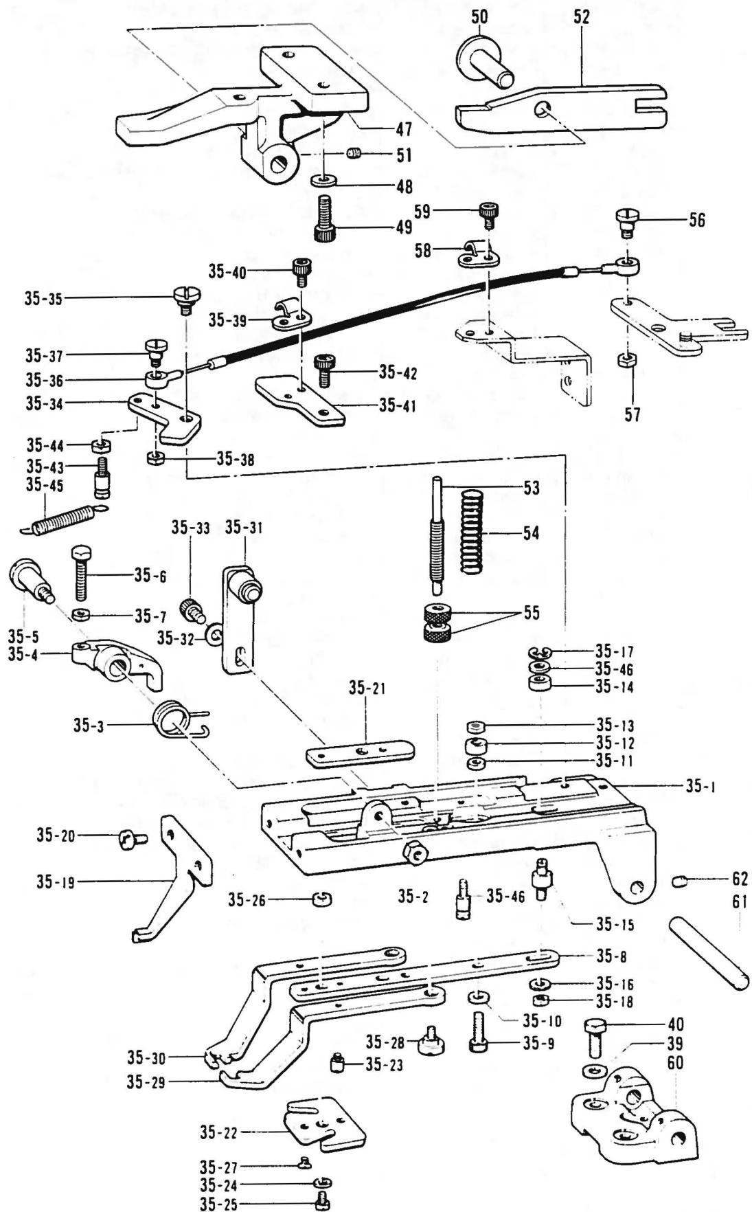
E2. 送り関係 /Feed mechanism/Transportvorrichtung/
