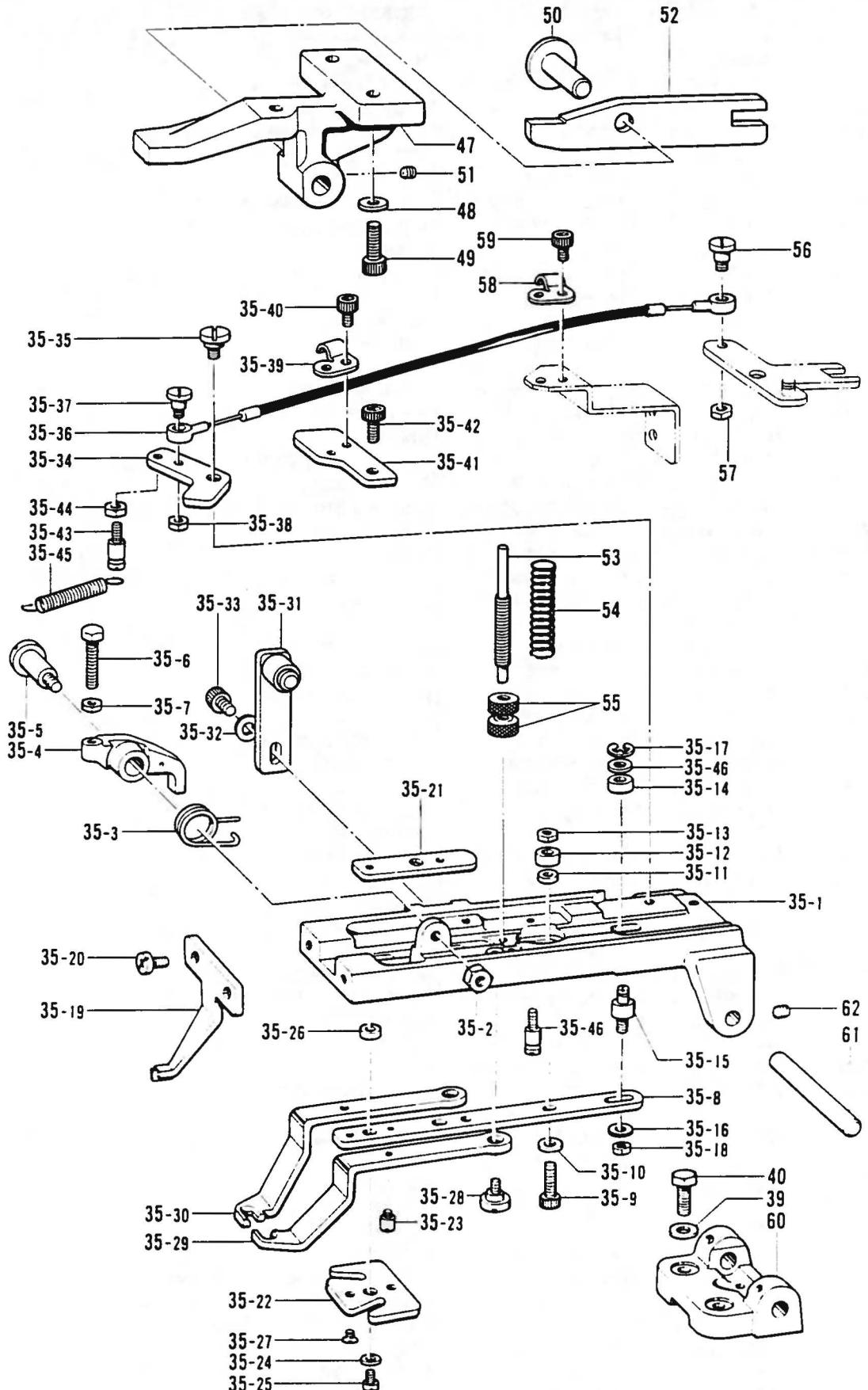
E2. 送り関係 / Feed mechanism / Transportvorrichtung /
